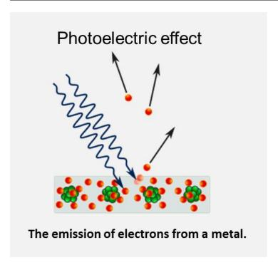
Light Photons are said to be absorbed by the electrons and energized electrons are projected out from metallic surfaces.
